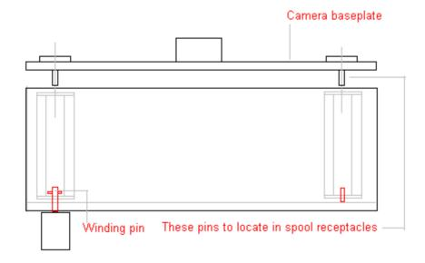
Close the back with the two base locking nuts and wind the film to exposure 2 as viewed in the red window located on the back of the camera
