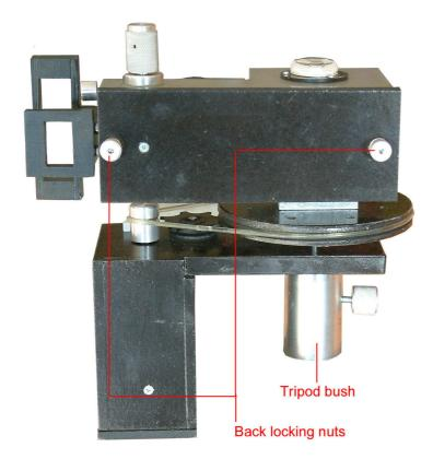
Remove the back of the camera by unscrewing the two Back locking nuts
