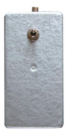
The switch is spring loaded to the centre position and the drive may be operated by pressing to the left or right..
