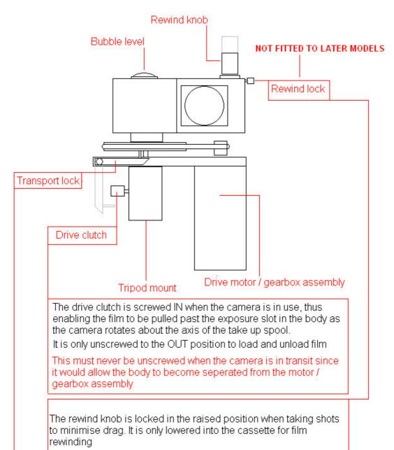
This is to be left in the locked position (as shown ) during transit to avoid pulling film through the camera. There are 8 holes in the main
