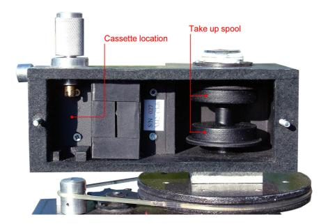
To load the cassette the rewind knob must be lifted upwards. It is the locked in this location by the rewind lock and left in this state since it eliminates another possible cause of friction when the film is being pulled out of the cassette.
