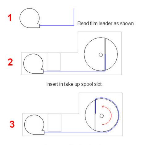
Rotate spool in direction shown for one turn to lock film in place
