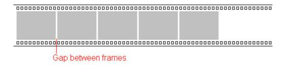
In a rotational, the concept of a discrete frame does not exist, the end of one shot and the start of another is as shown by a dense bar where the film was being continuously exposed when the camera was not rotating as shown below
